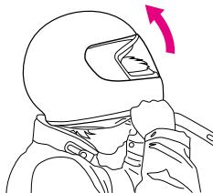
Undo a chinstrap first, and hold chinstraps by both hands. Spread the helmet apart by holding chinstraps, and remove a helmet from your head turning it backward as per Drawing.
