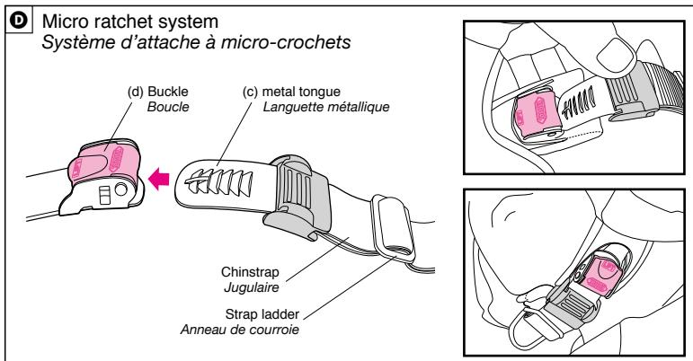
**Check that the chinstrap to ensure it is not loose:** The chinstrap should be as tight as possible without causing you pain. There must be no slack in the strap and it must be tight up against your chin. Correct tension in the chinstrap should allow normal breathing and swallowing but without leaving the space of a finger between the chinstrap and throat.
